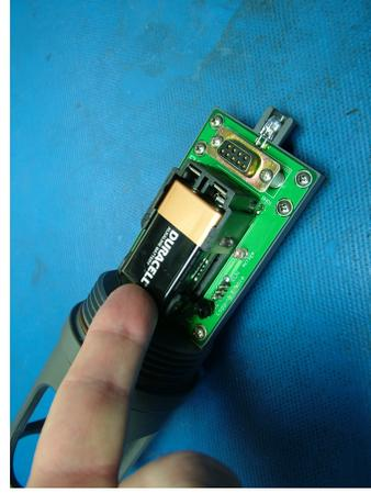
**Batteries will only seat when oriented correctly.
